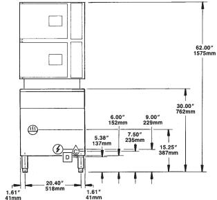
NOTE: When ordering optional reverse door openings: Control Panel, door openings, and cooking compartments are opposite that shown. Required clearance on left side, when ordered with reverse door openings, is 12.00" if adjoining wall or equipment is over 30.00" high.
